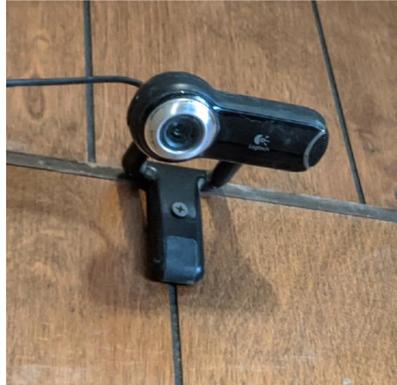
*Left: Because it is made to mount on the top edge of a laptop, provisions need to be made to mount it to a wall for use as a puppy cam. Thus the drilled hole in the middle of the mount for a wood screw. Right: Mounted eight feet off the floor, this camera can view a 6x8 floor area*
